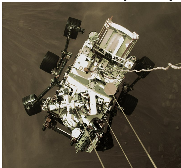
Perseverance being lowered to the Martian surface by the sky crane. Image Credit – NASA/JPL-Caltech
