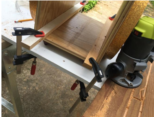
Figure 4: Preparing to cut notches for felt pads inside cradle
