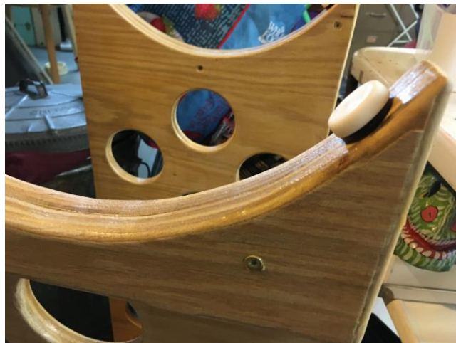
Figure 3: Plastic furniture pads for altitude trunnions
