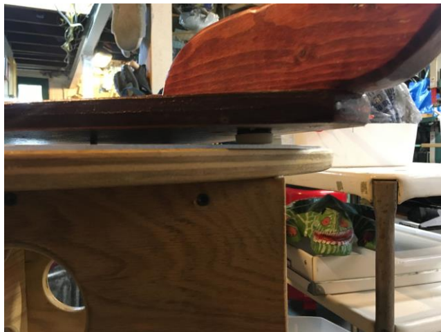
Figure 6: Upside down view of azimuth bearing and ground feet
