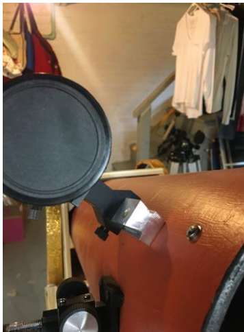
Figure 2: Hand-hewn rail for finder scope
